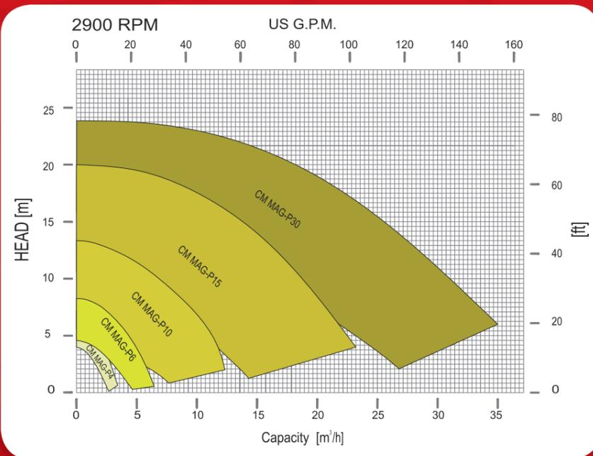
Pump construction and Operative Limits
