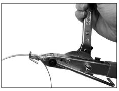
2. Form a clamp by threading the band through buckle and make a fold under the buckle. Insert tail of clamp into head of tool and slide into slot of winding mandrel. Depress locking pawl and tension clamp with forward strokes of the ratchet wrench.
