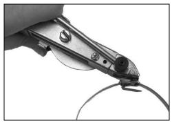
**3.** When sufficient tension has been applied, release locking pawl and rotate tool over object being clamped.
