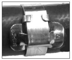
**5.** Complete clamping operation by tapping down ears of buckle with a hammer or mallet.
