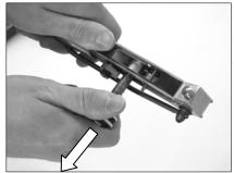
C) Tension the clamp with forward strokes of ratchet handle. When the desired tension is reached or the ratchet gear makes contact with the stop pin, release the ratchet handle. Tension will be maintained by the ratchet pawl.
